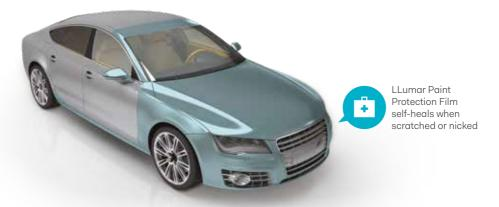
Self-healing occurs with application of moderate heat to the film (32° - 40° C). This can be induced by:
